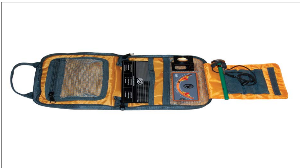
FIGURE 5.3: BCA snowpack observation tools including a thermometer, slope meter, loupe and snow crystal measuring card. SOURCE: < backcountryaccess.com >
